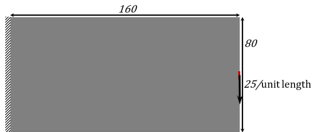
Fig. 20: Short cantilever fixed on the left edge and loaded on the center of right edge. Length of line of load = 8.
