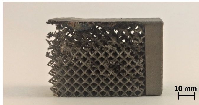
Figure 13: Using improper process parameters caused the lattice support structure to fail which led to the failure of the entire build. This example highlights the importance of manufacturability metric in support structure design.
