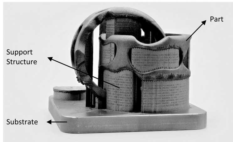
Figure 2: Stainless steel 316 object manufactured using SLM process. All overhanging surfaces are supported by a common support structure called block support (adopted from [18]).
