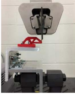
Figure 14: C-Bracket Fillet under compression. Test setup.
