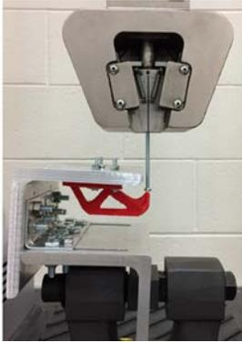
Figure 16: C-Bracket Fillet under Tension. Test setup.
