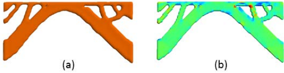
Figure 16: Final topology (a) and stress distribution (b) when the structure is subject to a spatially temperature gradient with resulting compliance and stress are as large as 4.17 and 1.98 times their initial values.
