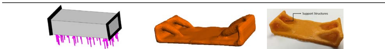
Figure 2: (a) Structural problem. (b) Optimized topology. (c) Fabricated part with support structures.
