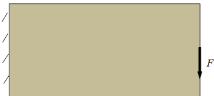
Figure 1: A single-load structural problem.
